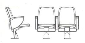
foundation expansion bolts M10 X 100 with washer and nut. Seat assembly made of Polyurethane foam moulded with 1.5 cm. thick water and termite proof plywood insert having effective seat width  $^{\sim}460.0$  mm and depth  $^{\sim}450.0$  mm. Polyurethane foam back assembly moulded with  $^{\sim}19$ mm x 16BG MS tubular frame insert. Stitched velvet finish fabric upholstery ( $^{\sim}400$  gm/running meter;
