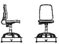
The seat and back should be of 1.2 cm. thick hot pressed water and termite proof plywood upholstered with fabric and moulded Polyurethane foam together with seat and back covers. The polyurethane foam moulded with density = 45 + -2 kg/m3 and Hardness = 20 + -2 on Hampden
